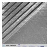
Figure 3. Deprocessed chip metal conductor lines.
