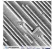
Figure 4. Deprocessed chip metal conductor lines.
