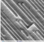
Figure 5. Deprocessed chip metal conductor lines, topographic shading image from Figure 4.
