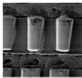
Figure 11. Etch defect resulting in non-through via.
