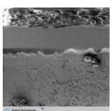
Figure 16. BGA contact pad, board contact interface.
