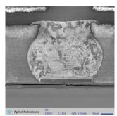
Figure 15. BGA contact pad.
