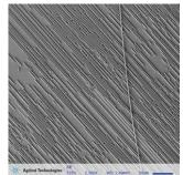
Figure 1. Deprocessed chip metal conductor lines.
