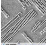
Figure 2. Deprocessed chip metal conductor lines.
