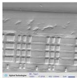
Figure 9. Etch defect resulting in non-through via, topographic shading image.
